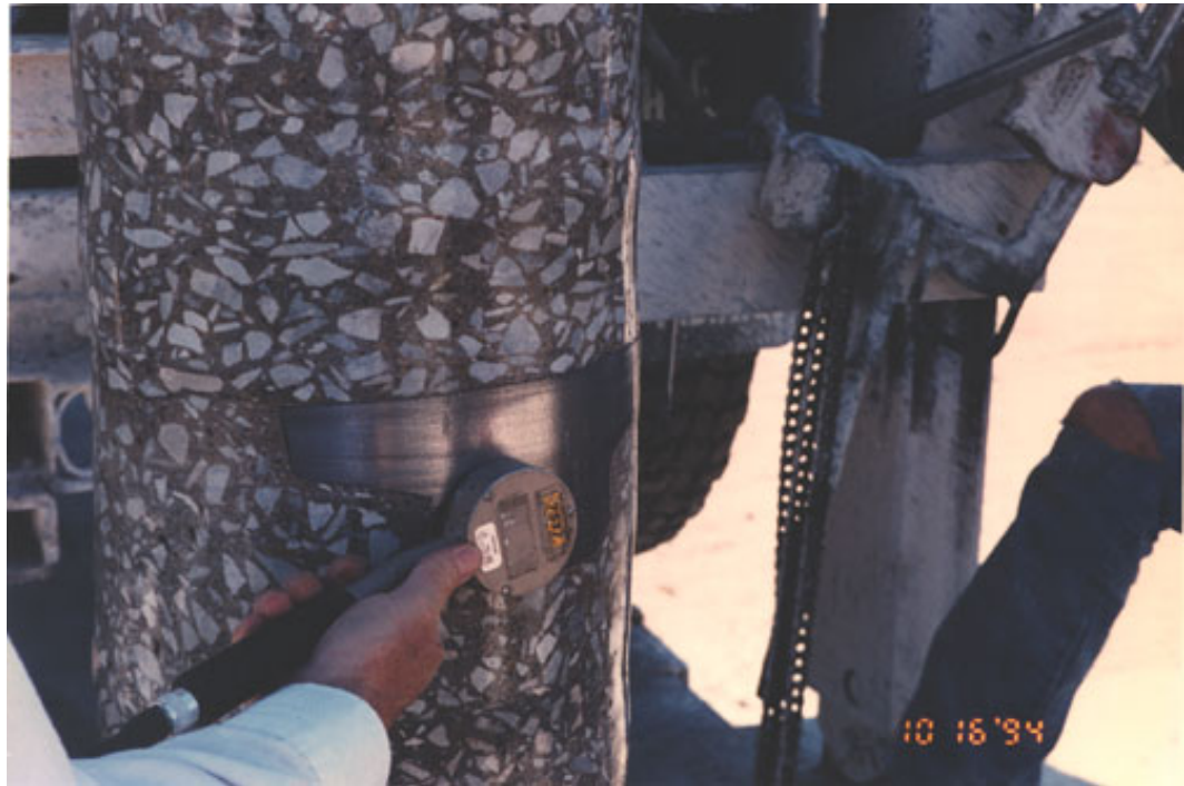
Figure 3-18 Core Drill Contact with End Cap
