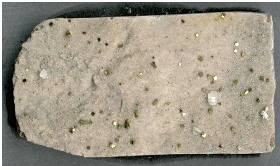
Figure 10 Calcite and pyrite crystals on top of a quartz coated fracture surface. Length of photograph is 2.5 cm (KFM01A 267.0 m). From Sandström et al. [20].
