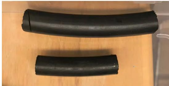
Figure 25 shows the EPDM reference O-ring, which has been used for comparing to the cable samples provided by Ringhals and Forsmark.
