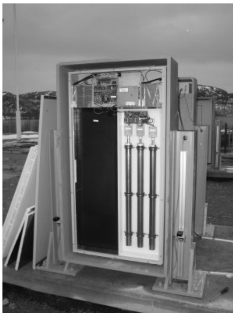
Figure 1. One of the detector modules without its cover; the modules contain a PVC scintillator for gamma ray measurements and three helium tubes for neutron detection (Photo: NRPA).
