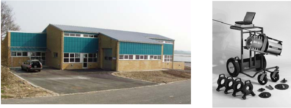
Figure 1. Clearance laboratory at the Risø-site placed close to Roskilde Fjord away from the nuclear facilities. The laboratory is equipped with two germanium detectors with lead collimators.
