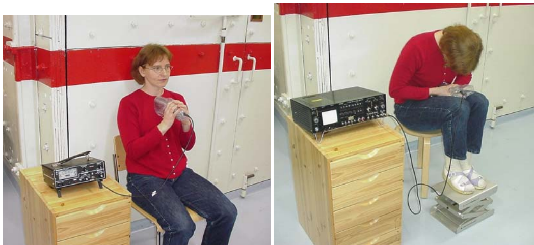
Figure 1 Left: Thyroid measurement with a hand-held instrument based on a NaI(Tl)-detector. Right: A rapid whole-body measurement with similar instrument.
