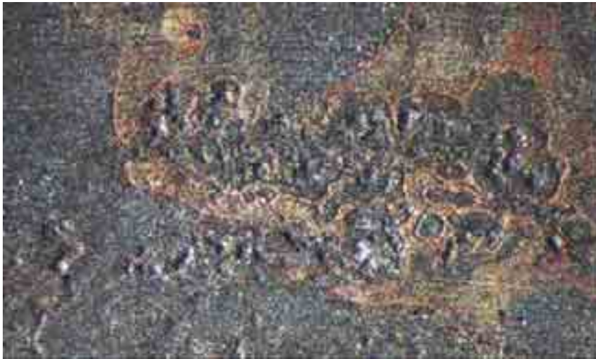
Figure 3 LOM photograph taken in an area with small whisker roots. The horizontal length of the picture covers 2.5 mm.
