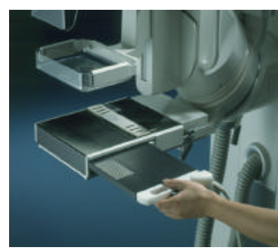
Figure 8. A CsI(Tl)-CCD detector with a 4.9 cm x 8.5 cm field of view. The principle of operation is shown (left) as well as the use of the detector in a cassette that can replace a film cassette in a mammography unit (right). (Figures supplied by Siemens).
