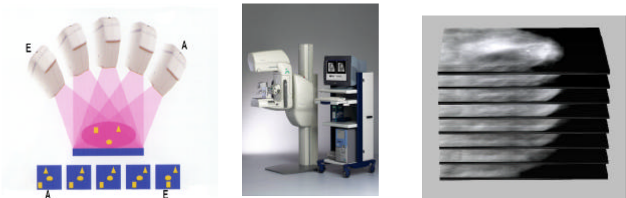
Figure 14. The principle of tomosynthesis (left), the Instrumentarium tomosynthesis mammography system Delta 32 TACT (middle) and an example of reconstructed images from that system (right). (Figures supplied by General Electric (left) and Instrumentarium Imaging).
