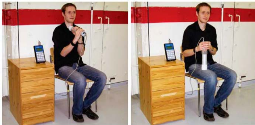
Figure 1: Illustration for thyroid (C) and corresponding body background (CB) measurement, as recommended in TMT handbook (Rojas-Palma 2009)
