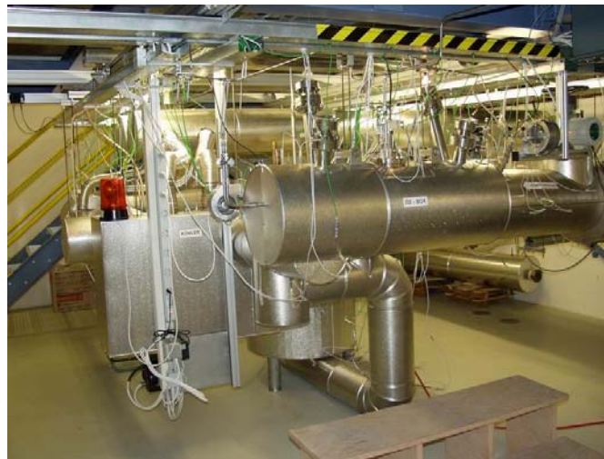
Figure 9: The Karlsruhe Lead Laboratory – KALLA. A part of the Pb-Bi loop.
