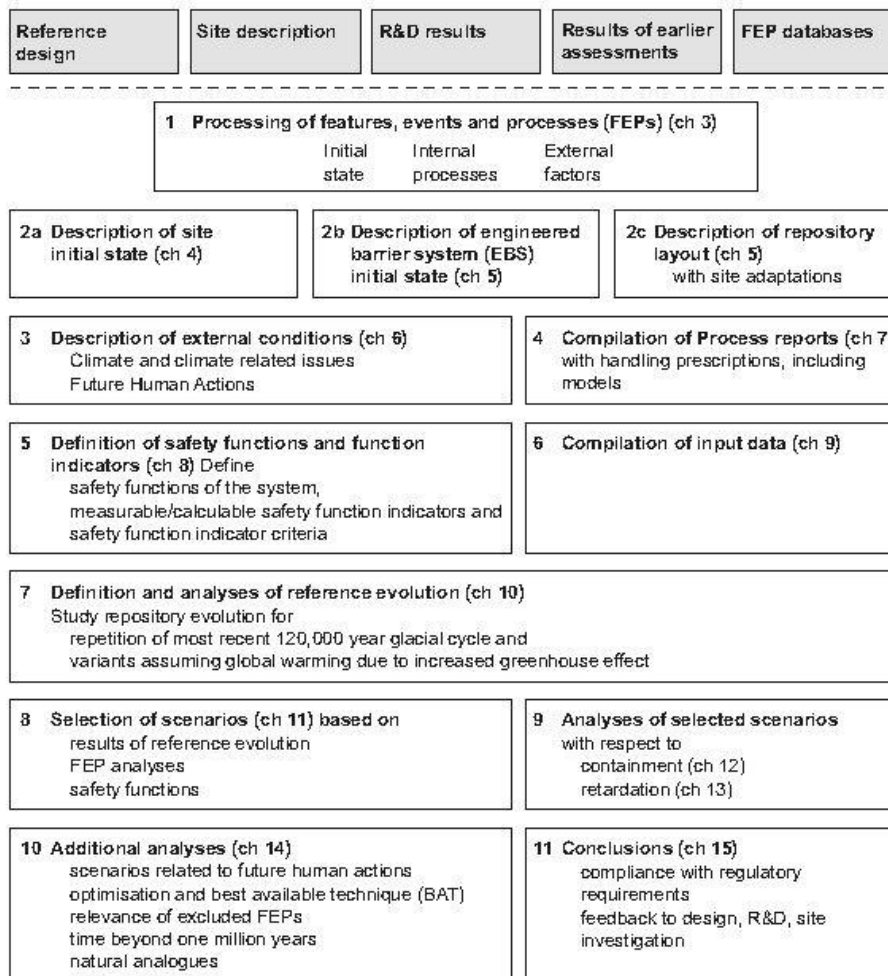
Figure 1.3: An outline of the eleven main steps of the SR-Site safety assessment. The boxes at the top above the dashed line are inputs to the assessment. The chapters in the main report where the steps are further documented are also indicated (TR-11-01 S-6: references given in the figure refer to report SKB TR-11-01).
