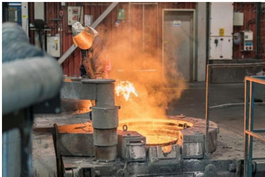
Figure 11. Radioactive scrap metal volume reduced by melting within the metal treatment facility SMA [18].
