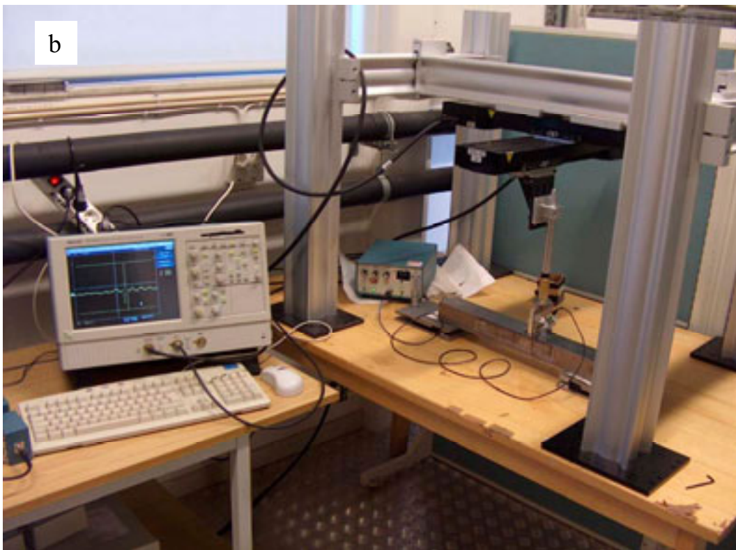
Figure 1: a) detailed view of a steel beam and transducer holder; b) overview of the experimental set up.
