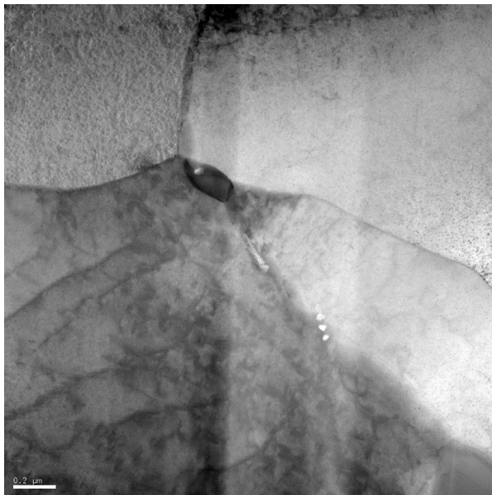
Figure 24 TEM bright field image of an area including precipitates in the grain boundaries.
