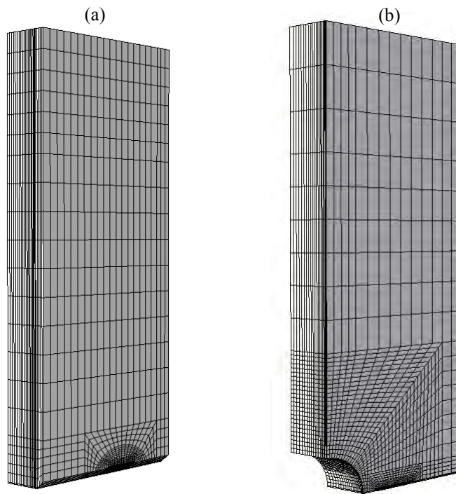
Figure 5.3. Three dimensional finite element mesh for (a) a quarter model of the side-grooved three point bending specimen, (b) a quarter model of the un-grooved notched three point bending specimen.
