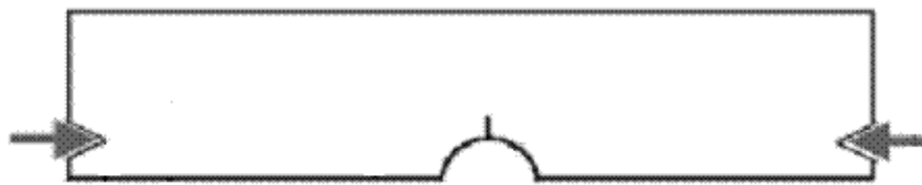
Figure 5.16. In-plane compression of notched test specimen.
