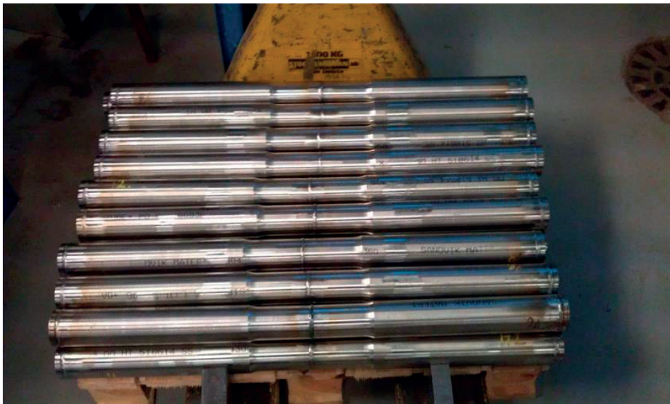
(b) Different test specimens after welding and prior to undergoing fatigue testing.
