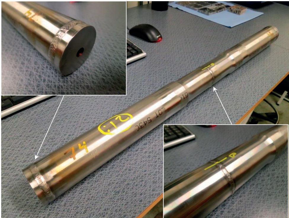
(a) Close-up views of the performed butt welds on a finished test specimen.
