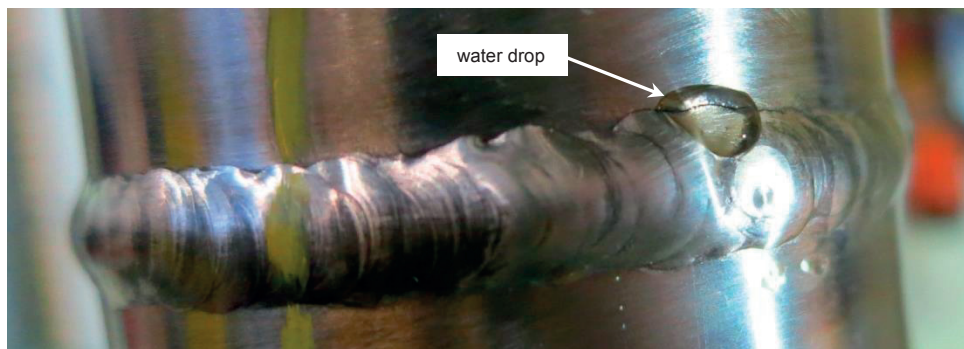
Figure 14. Illustration of visual detection of onset of leakage during final stage of fatigue testing.
