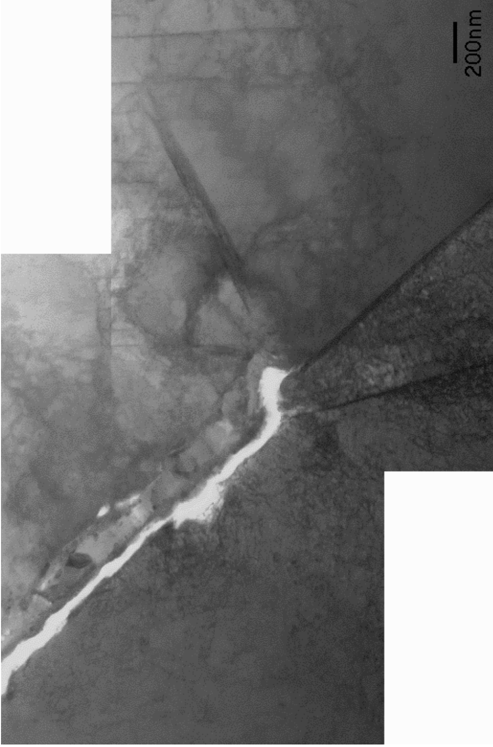
Figure 10: Montage of electron micrographs showing crack tip propagating along grain boundary
